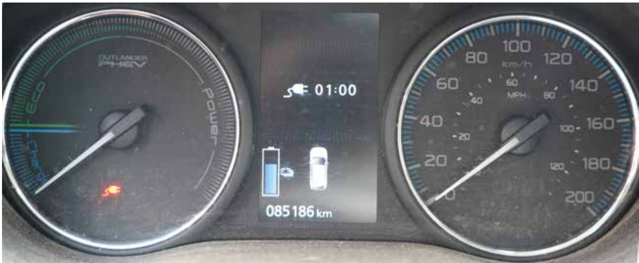
▲ Dashboard screen showing the charging progress for a plug-in hybrid. At the top of the left circle, the PHEV stands for plug-in hybrid electric vehicle. The red light at bottom indicates that the car is plugged in.
