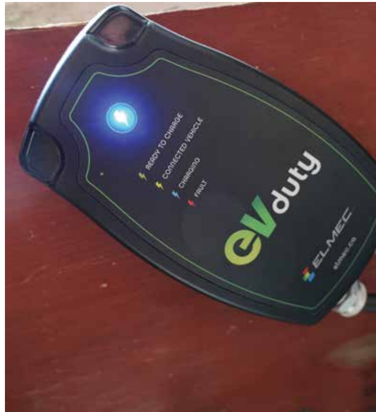
▼ Level 2 home charger in use. This requires the 240-volt household connection.
