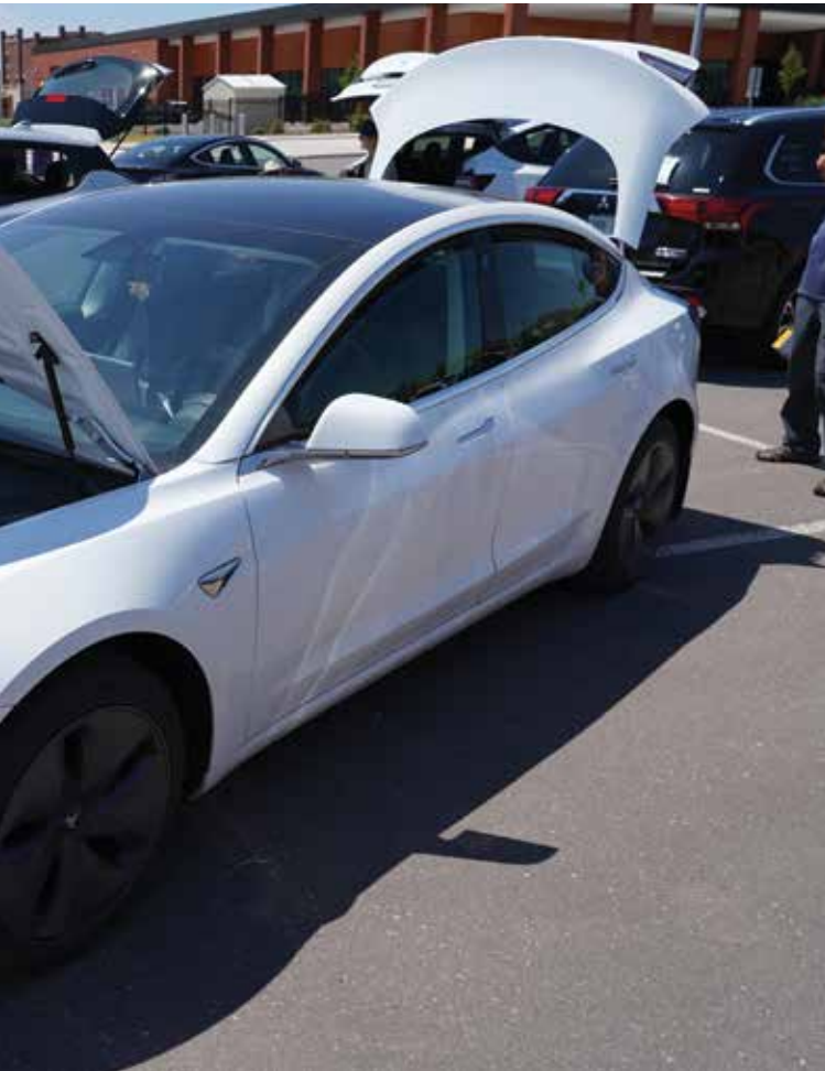
▲ Storage in an EV can be available under the front hood as well as in the rear trunk. The engine and battery tend to be less visible in EVs.
