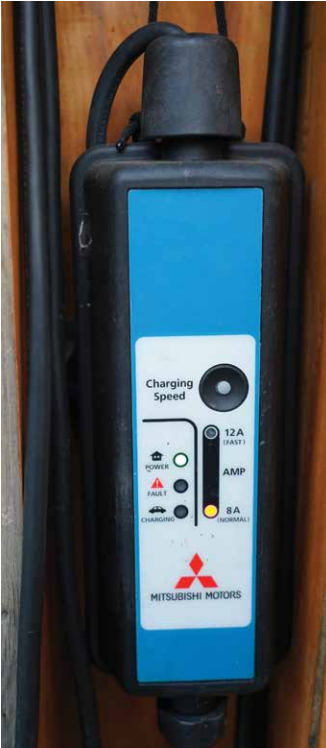
◀ Level 1 home charger. This slowest charger comes with the car and can be plugged into a 120-volt, three-pronged outlet.
