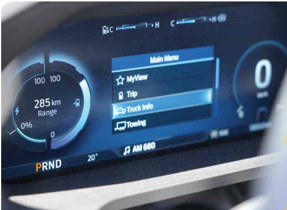
◀ Remaining range of distance available from the battery, shown on a dashboard.
