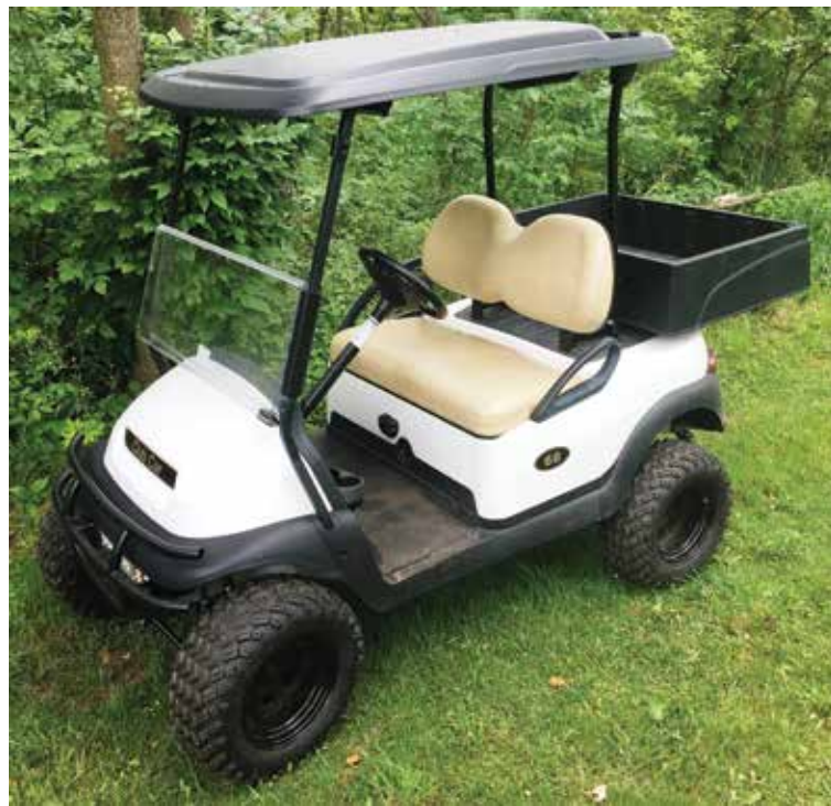
The customized golf car with raised base, heavy-duty tires and cargo box. PHOTO BY MIKE DAVIS.
