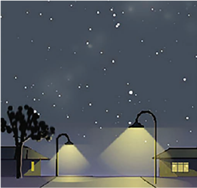
▲ Preventing upward light spill from fixtures keeps illumination low and helps prevent light pollution. ILLUSTRATION PROVIDED.
